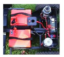
Connect the batteries ensuring that all connections are secure.
