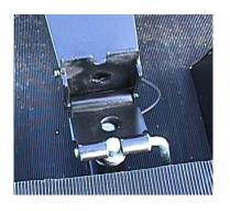
Hold the lever "B" horizontal then drop the thumbscrew "A" into the slot and tighten it.
